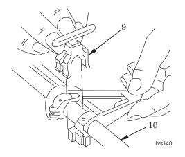
Figure 6. Removal/Installation of Swivel Mount (Carbine).
