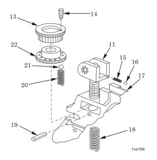
Figure 4. Disassembly of Rear Sight Assembly.
