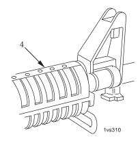
Figure 6. Attaching Sling to Top Sling Adapter and Clamp.
