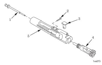
Figure 10. Assembly of Bolt and Bolt Carrier Assembly.
