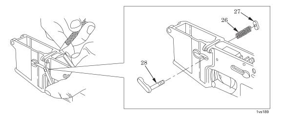
Figure 21. Installation of Magazine Catch.
