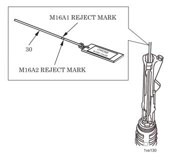
Figure 32. Use of Barrel Erosion Gage.
