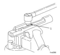
Figure 3. Torquing Carrier Key Screws.
