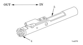
Figure 7. Checking for Binding of Bolt Assembly.
