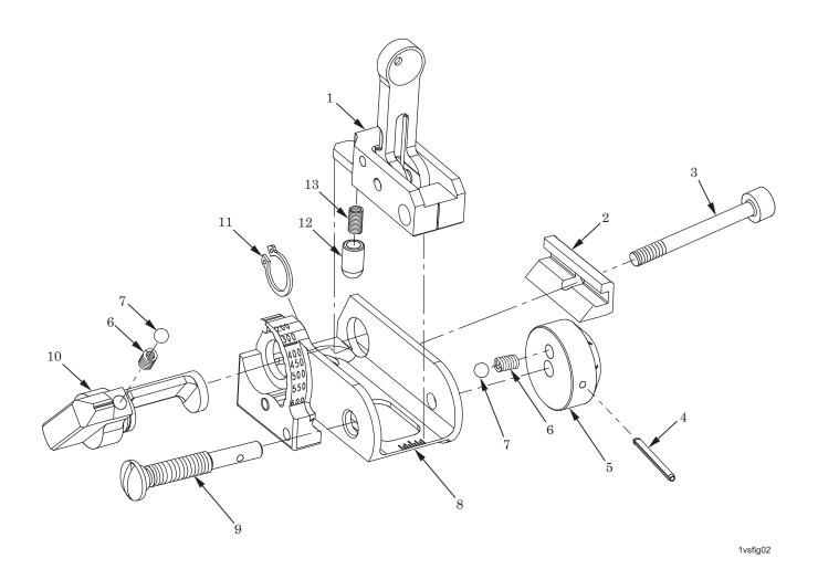
Figure 2. Back-up Iron Sight Assembly (M16A3, M16A4, M4, M4A1) 12996812.
