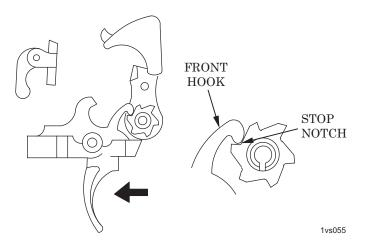
Figure 4. Firing of First Round.
