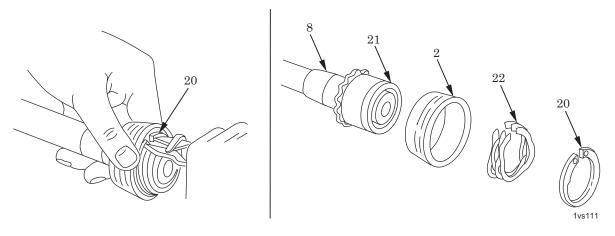
Figure 18. Installation of Handguard Slip Ring.
