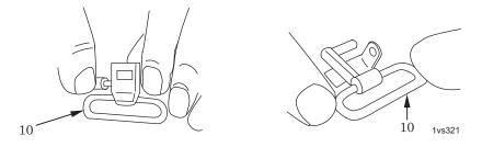
Figure 10. Attaching Swivel to Lanyard.
