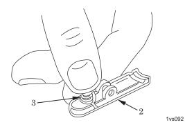
Figure 12. Installation of Extractor Spring Assembly.
