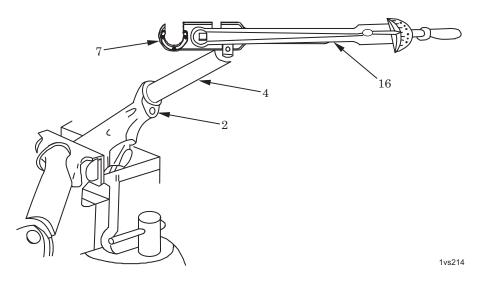
Figure 8. Torquing Lower Receiver Extension (Rifle).
