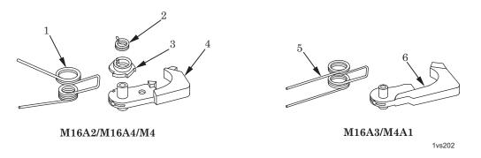
Figure 1. Disassembly of Hammer Assembly.
