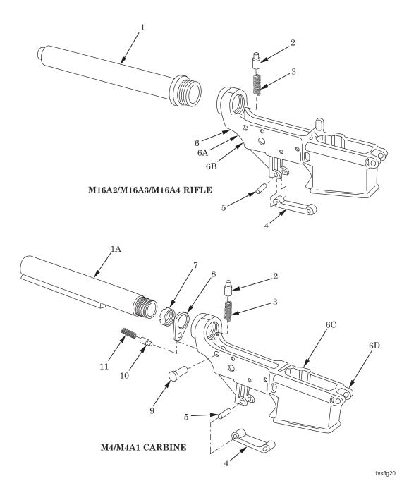
Figure 20. Lower Receiver and Receiver Extension Assembly (M16A2) 9349101, (M16A3) 12012002, (M16A4) 12598102, (M4) 9390011, and (M4A1) 12972690.
