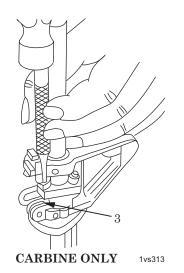
Figure 2. Removing Two Spring Pins.
