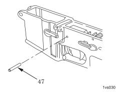
Figure 28. Hammer Pin Inspection.
