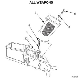
Figure 28. Installation of Pistol Grip.
