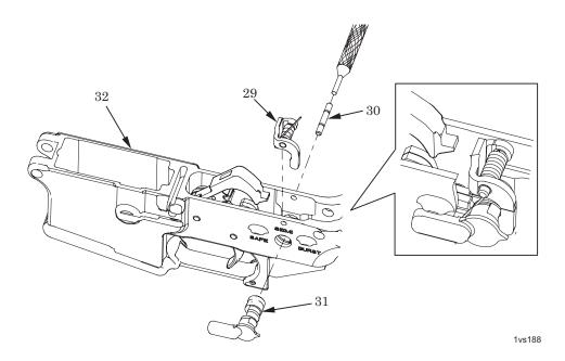
Figure 20. Installation of Sear and Selector Lever.
