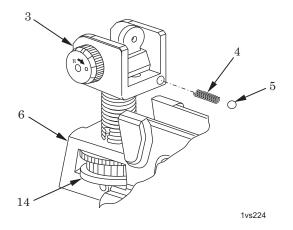
Figure 4. Installation of Rear Sight Assembly.
