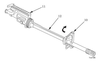
Figure 6. Removal of Gas Tube.
