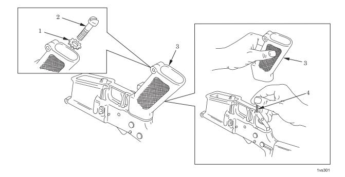
Figure 5. Removing Pistol Grip for Lock Plate Removal.
