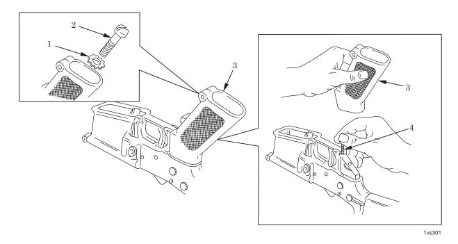
Figure 1. Removing Pistol Grip for Lock Plate Installation.
