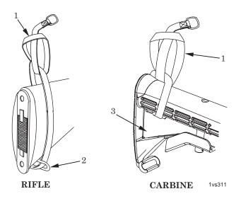
Figure 7. Removing Top Sling Adapter.
