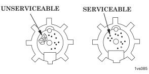
Figure 5. Bolt Face Inspection.
