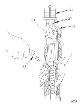
Figure 36. Use of Weights in Headspace Check.
