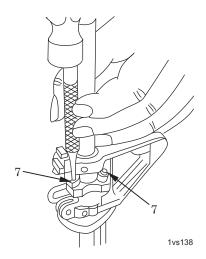
Figure 4. Removal/Installation of Spring Pins (Carbine).
