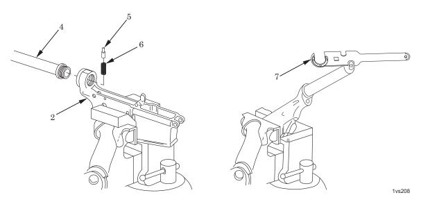
Figure 2. Removal of Lower Receiver Extension (Rifle).
