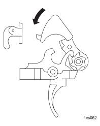
Figure 17. Final Movement of Key and Bolt Carrier Assembly.
