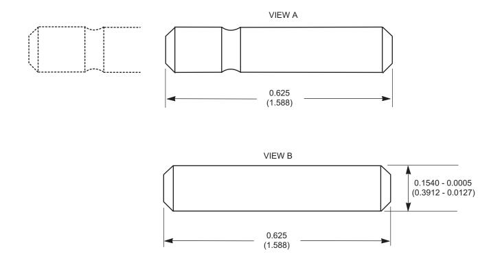
FABRICATE FROM OLD TRIGGER PIN (VIEW A) PN8448609 OR FABRICATE SLAVE PIN (VIEW B) FROM MATERIAL BLOCK, WIRE, STEEL ALLOY, GRADE 4140, ASTM-A547 OR EQUIVALENT.
