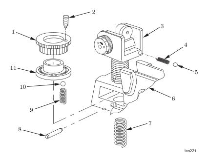
Figure 1. Disassembly of Carrying Handle Assembly.
