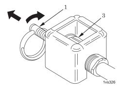
Figure 4. Unscrewing Slide from Compensator.
