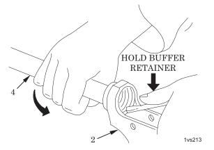
Figure 7. Installation of Lower Receiver Extension (Rifle).
