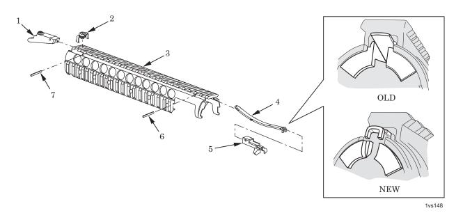
Figure 2. Disassembly/Assembly of Handguard Assembly.
