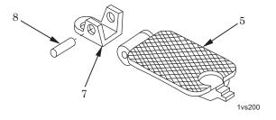
Figure 3. Disassembly/Assembly of Door Assembly.
