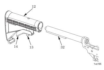
Figure 27. Installation of Buttstock Assembly (Carbine).
