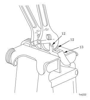
Figure 2. Straightening Rear Sight Guards.
