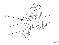
Figure 20. Barrel Gas Port Cleaning.
