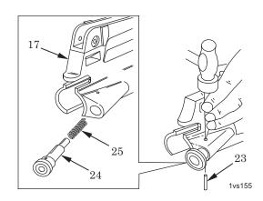
Figure 5. Removal of Forward Assist Assembly.
