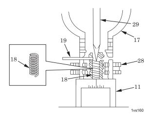
Figure 10. Installation of Helical Spring.
