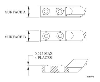
Figure 4. Inspection of Carrier Key Screws.
