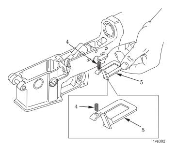
Figure 6. Removing Lock Plate.
