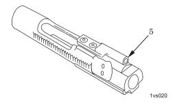
Figure 18. Bolt Carrier Key Inspection.
