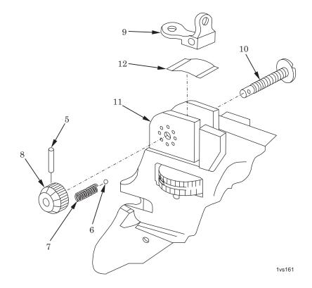
Figure 11. Installation of Sight Aperture and Windage Knob.
