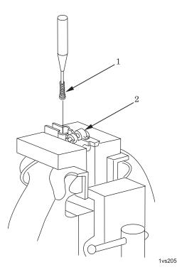
Figure 2. Installation of Disconnector Springs (M16A2/M16A4/M4).
