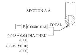
FABRICATE FROM 0.245 IN. STEEL AISI 1095 OR EQUIVALENT. HARDEN AND TEMPER TO RC 57-61 FOR LENGTH -A-FINISH: NO. 5.3.1.2 OR 5.3.2.2 OF MIL-STD-171.
