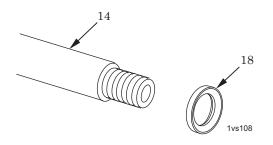
Figure 8. Removal of Recessed Washer.
