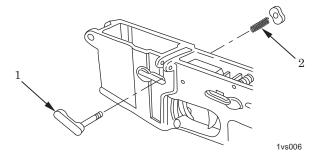
Figure 1. Magazine Catch Inspection.
