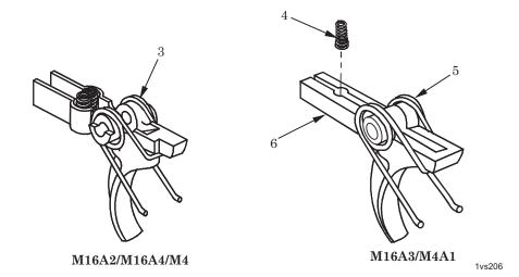
Figure 3. Installation of Trigger Spring.
