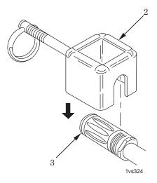
Figure 2. Placing Blank Firing Attachment.
