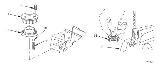
Figure 3. Assembly and Installation of Elevation Knob Assembly.
