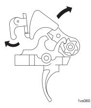
Figure 9. Forward Travel of Key and Bolt Carrier Assembly.
