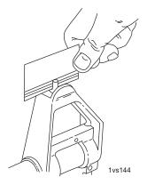
Figure 10. Measurement of Height of Front Sight Post.
