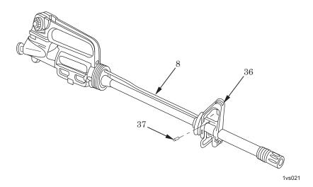
Figure 19. Adjustment of Gas Tube.
