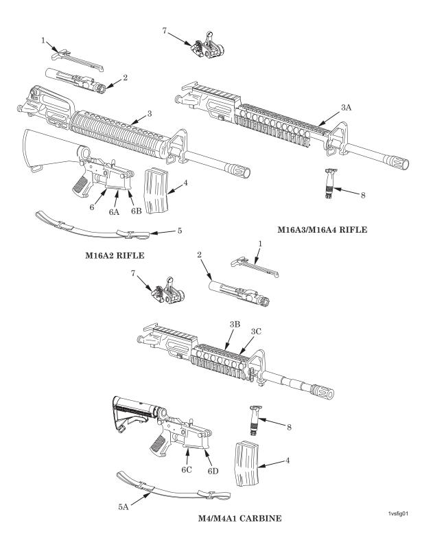
Figure 1. Rifle, 5.56mm (M16A2) 9349000; Rifle, 5.56mm (M16A3) 12012000; Rifle, 5.56mm (M16A4) 12973001; Carbine, 5.56mm (M4) 9390000; and Carbine, 5.56mm (M4A1) 12972700.
