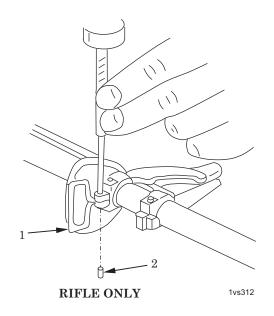
Figure 1. Removing Sling Swivel.
