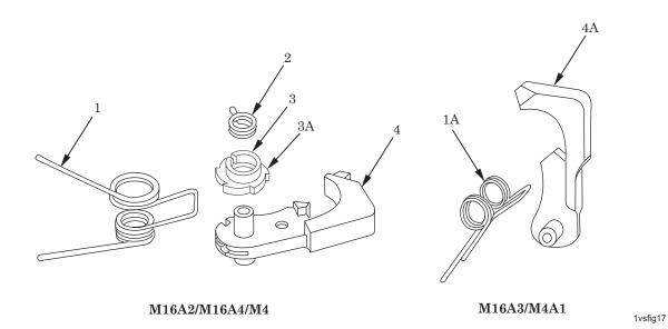
Figure 17. Hammer Assembly (M16A2, M16A4) 9349106, (M4) 9390032, and (M16A3, M4A1) 8448610.
