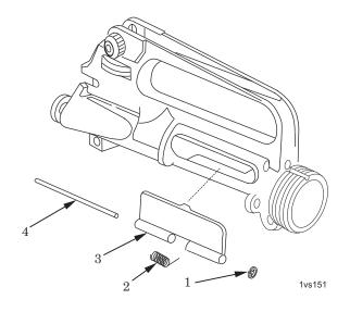
Figure 1. Removal of Ejection Port Cover.
