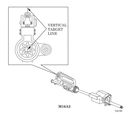
Figure 21. Alignment of Front and Rear Sights.
