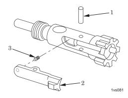
Figure 1. Removal of Cartridge Extractor.
