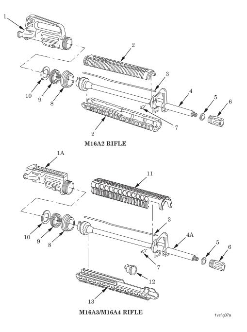
Figure 7. Upper Receiver and Barrel Assembly (M16A2) 9349050, (M16A3, M16A4) 12973010, and (M4, M4A1) 12972680 (Sheet 1 of 2).
