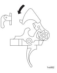
Figure 11. Rearward Movement of Key and Bolt Carrier Assembly.
