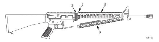
Figure 3. Removal of Upper and Lower Handguards (M16A3/M16A4/M4/M4A1).
