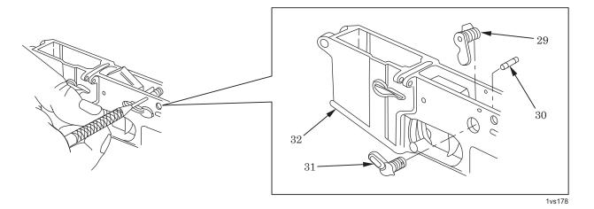
Figure 10. Removal of Sear and Selector Lever.
