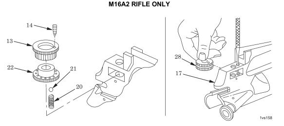
Figure 8. Assembly and Installation of Elevation Knob Assembly.
