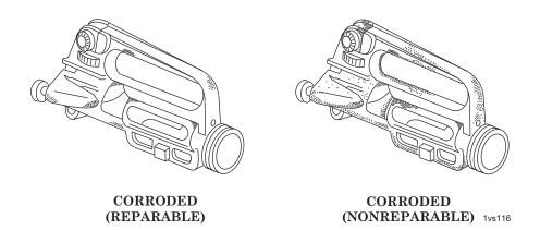
Figure 16. Inspection for Corrosion.
