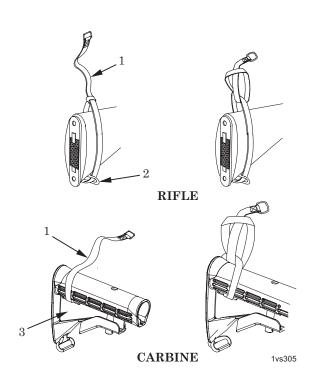
Figure 1. Installing Top Sling Adapter.
