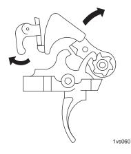
Figure 15. Release of Hammer Assembly.
