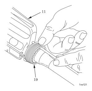
Figure 22. Alignment of Barrel Nut Assembly.
