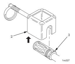
Figure 5. Removing Blank Firing Attachment.
