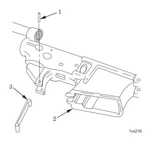
Figure 10. Installation of Trigger Guard.
