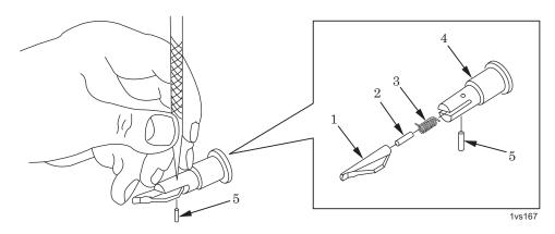
Figure 1. Disassembly of Forward Assist Assembly.
