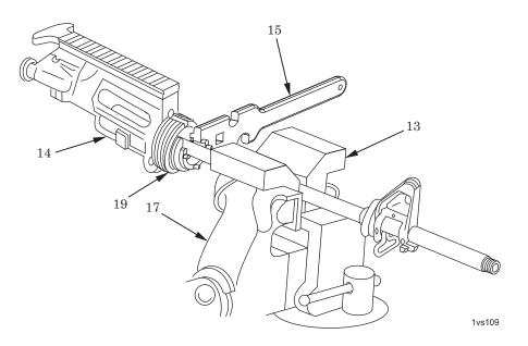
Figure 9. Loosening of Barrel Nut Assembly.
