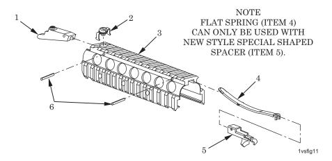
Figure 11. Upper Handguard Assembly (M4, M4A1) 12973096.
