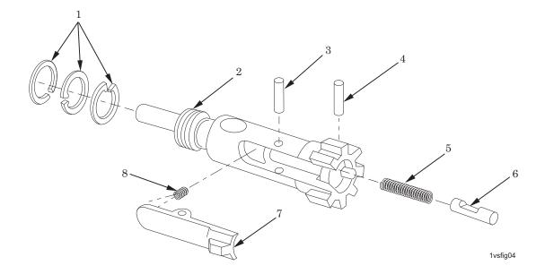
Figure 4. Breech Assembly Bolt 13004787.
