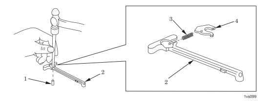
Figure 1. Disassembly of Charging Handle Assembly.
