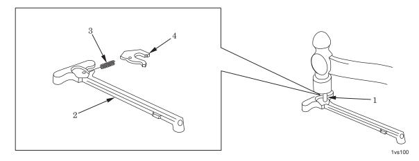
Figure 2. Assembly of Charging Handle Assembly.
