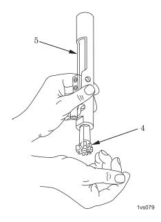
Figure 8. Checking for Fit of Bolt Assembly.
