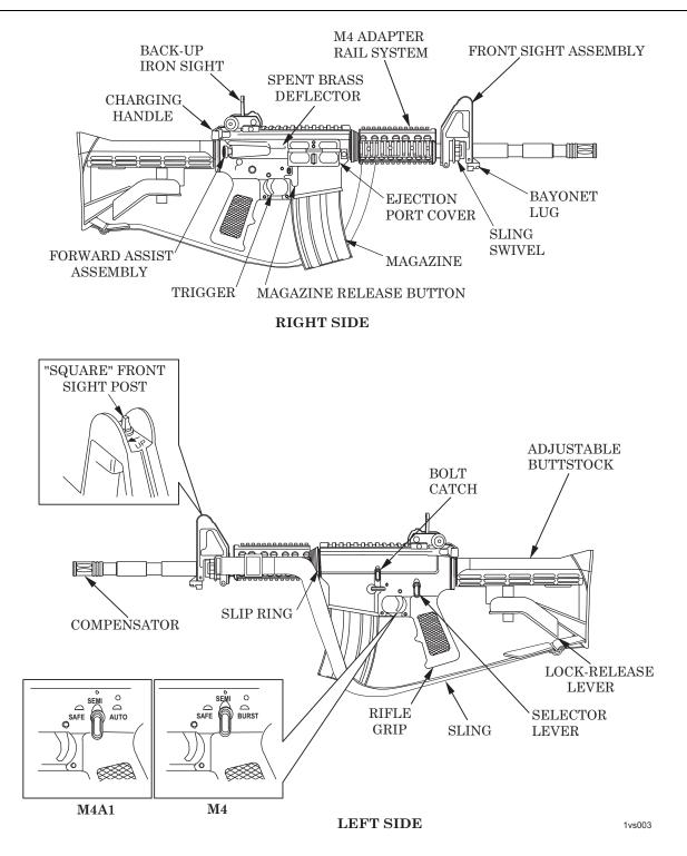
Figure 3. External View of 5.56mm Carbine, M4/M4A1.
