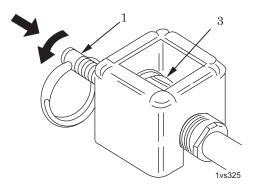
Figure 3. Securing Blank Firing Attachment.
