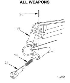
Figure 7. Installation of Forward Assist Assembly.
