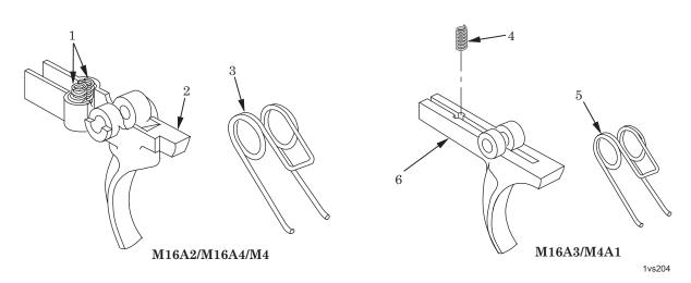
Figure 1. Disassembly of Trigger Assembly.
