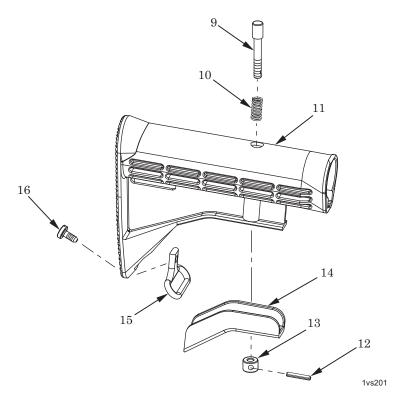
Figure 4. Disassembly/Assembly of Buttstock Assembly (Carbine).
