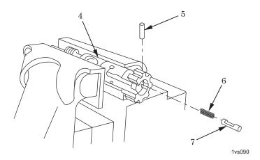
Figure 10. Installation of Cartridge Ejector.
