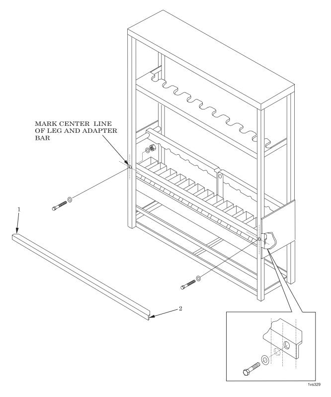
Figure 1. Installing Adapter Bar on M12 Storage Rack.
