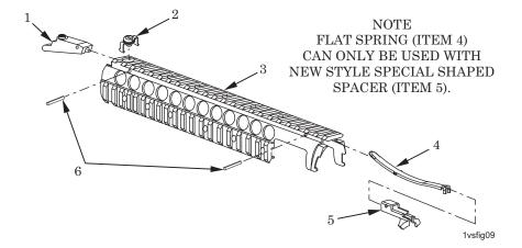
Figure 9. Upper Handguard Assembly (M16A3, M16A4) 12973021.
