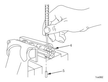
Figure 2. Removal of Spring Pin.
