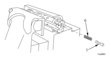
Figure 3. Removal of Cartridge Ejector.
