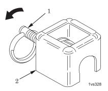
Figure 6. Securing Slide in Blank Firing Attachment.
