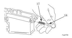
Figure 6. Removal of Detent and Helical Spring.
