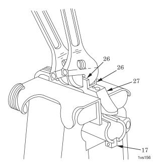
Figure 6. Straightening Rear Sight Guards.
