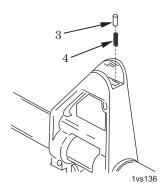
Figure 2. Removal/Installation of Front Sight Detent and Spring.
