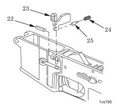
Figure 22. Installation of Bolt Catch.
