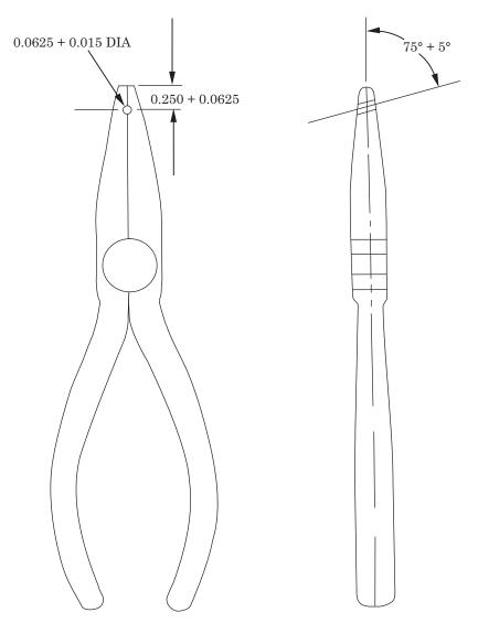
FABRICATE FROM NEEDLE NOSE PLIERS, NSN 5120-00-268-3579 OR EQUIVALENT.
