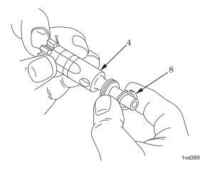
Figure 9. Installation of Bolt Rings.
