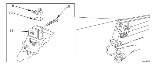
Figure 3. Removal of Sight Aperture.
