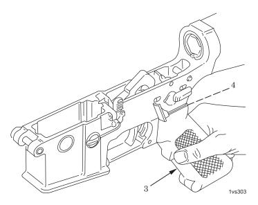
Figure 3. Positioning Pistol Grip with Lock Plate Installed.
