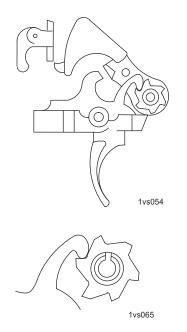
Figure 19. Rotation into Stop Notch.
