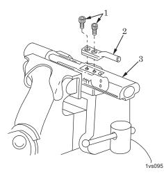
Figure 2. Installation of Carrier Key.
