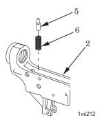
Figure 6. Installation of Buffer Retainer (Rifle).
