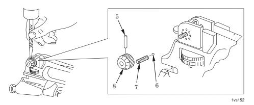
Figure 2. Removal of Windage Knob.
