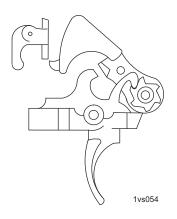
Figure 3. Beginning Position in Three-Round Burst.
