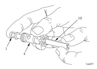
Figure 6. Firing Pin Protrusion Test.
