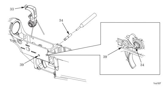
Figure 19. Installation of Hammer Assembly.
