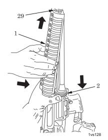
Figure 30. Installation of Upper Handguard Assembly (M16A2).
