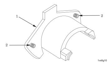
Figure 10. Barrel Stop Assembly (M16A3, M16A4) 12973139.
