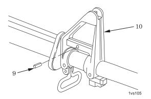
Figure 5. Removal of Spring Pin.
