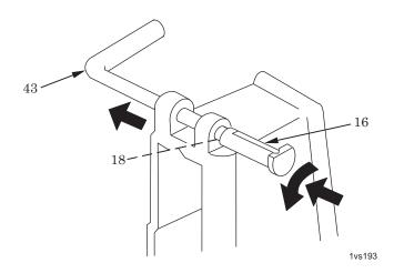
Figure 25. Installation of Pivot Pin.
