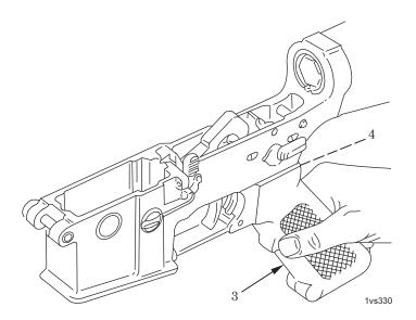
Figure 7. Positioning Pistol Grip with Lock Plate Removed.
