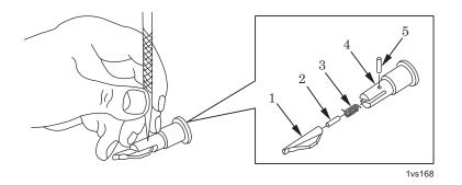
Figure 2. Assembly of Forward Assist Assembly.
