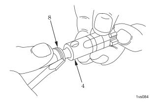
Figure 4. Removal of Bolt Rings.
