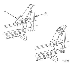
Figure 5. Removing Clamp from Front Sight.
