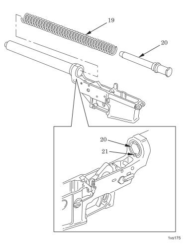
Figure 7. Removal of Buffer Assembly and Action Spring.
