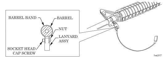
Figure 6. Attaching Lanyard Assembly.
