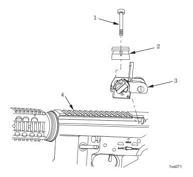
Figure 1. Removal of Back-up Iron Sight.
