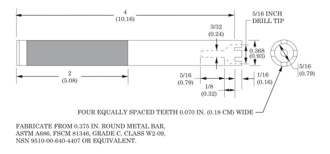
NOTES: 1. ALL DIMENSIONS SHOWN ARE IN INCHES WITH METRIC CONVERSION TO CENTIMETERS IN PARENTHESES. 2. TEETH MUST BE HAND FILED TO FIT FRONT SIGHT POST.
