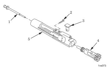
Figure 1. Disassembly of Bolt and Bolt Carrier Assembly.
