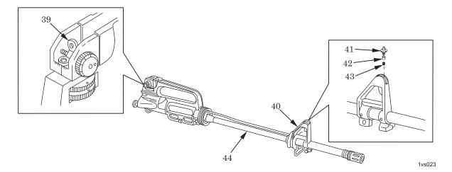
Figure 21. Front Sight and Rear Sight Inspection.
