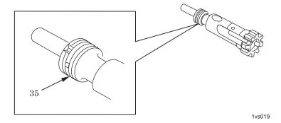
Figure 17. Bolt Ring Gap Adjustment.
