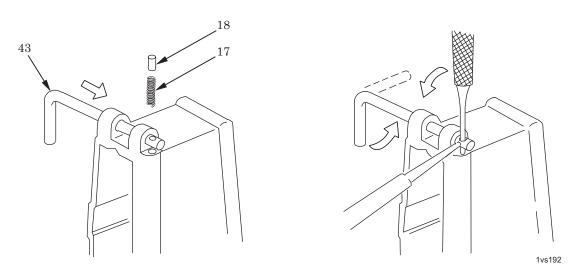
Figure 24. Installation of Pivot Pin Detent.
