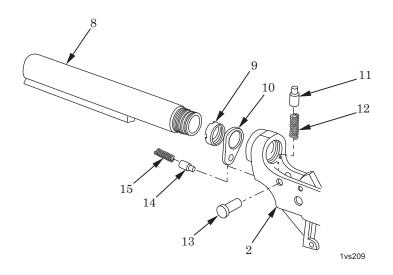
Figure 3. Removal of Lower Receiver Extension (Carbine).
