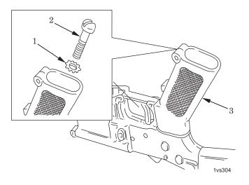
Figure 4. Securing Pistol Grip with Lock Plate Installed.
