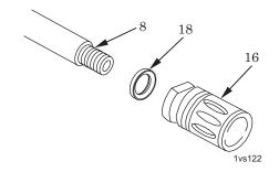
Figure 23. Installation of Compensator.
