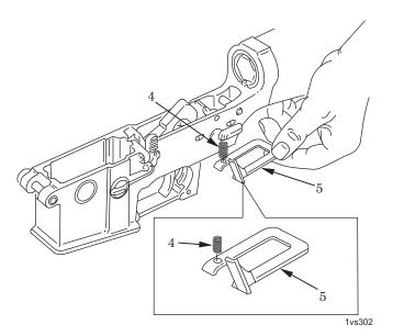
Figure 2. Installing Lock Plate.
