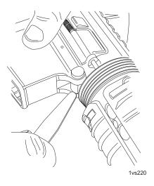
Figure 29. Use of Thickness Gage.
