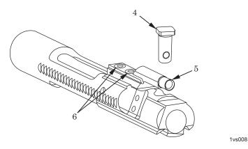
Figure 4. Bolt Carrier Assembly Inspection.
