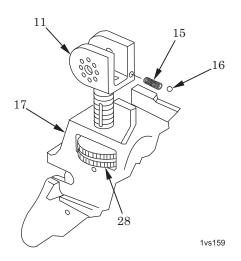
Figure 9. Installation of Rear Sight Base.
