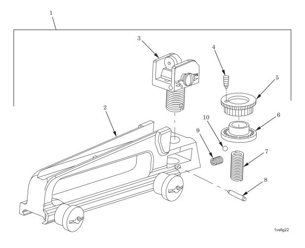
Figure 22. Carrying Handle Assembly (M16A3, M16A4, M4, M4A1) 12951011.
