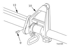
Figure 26. Installation of Spring Pin.
