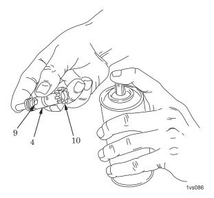
Figure 6. Inspection for Cracks in Bolt Assembly.
