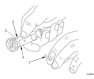
Figure 13. Installation of Extractor Pin.
