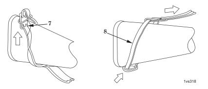
Figure 7. Attaching Rear Sling Adapter.
