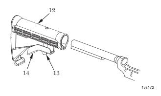
Figure 4. Removal of Buttstock Assembly (Carbine).
