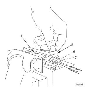
Figure 11. Installation of Spring Pin.
