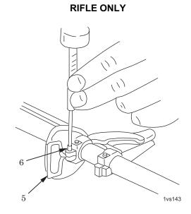
Figure 9. Installation of Small Sling Swivel (Rifle).
