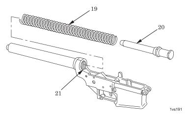
Figure 23. Installation of Action Spring and Buffer Assembly.
