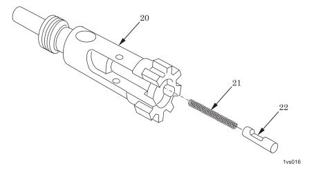
Figure 13. Cartridge Ejector Inspection.
