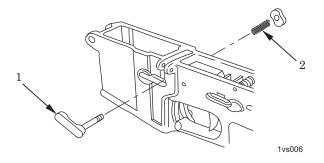
Figure 2. Magazine Catch and Spring Inspection.
