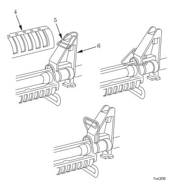
Figure 2. Installing Clamp on Front Sight.
