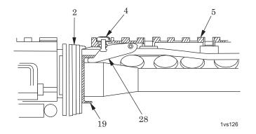
Figure 28. Installation of Upper Handguard Assembly (M16A3/M16A4/M4/M4A1).
