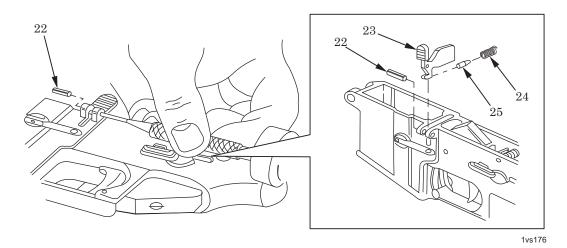
Figure 8. Removal of Bolt Catch.
