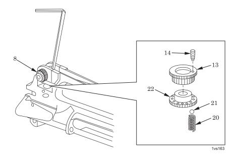
Figure 13. Zeroing Elevation Knob.
