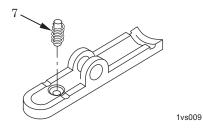
Figure 5. Extractor Spring Assembly Inspection.
