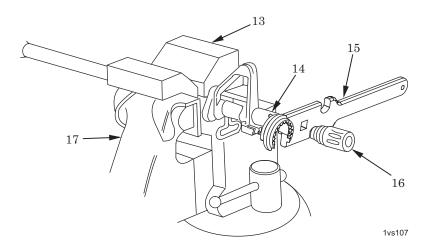
Figure 7. Removal of Compensator.
