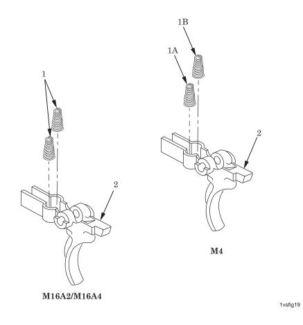
Figure 19. Trigger Subassembly (M16A2, M16A4) 9392518 and (M4) 12972696.
