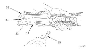
Figure 34. Insertion of Headspace Gage.
