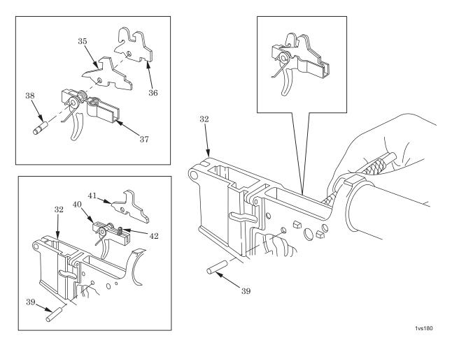
Figure 12. Removal of Trigger Assembly.
