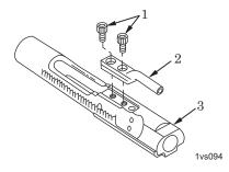
Figure 1. Disassembly of Key and Bolt Carrier Assembly.
