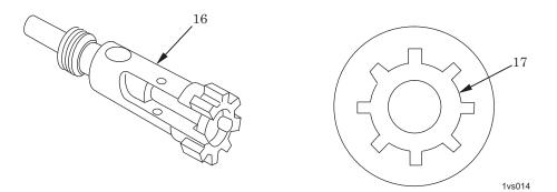
Figure 11. Locking Lugs Inspection.
