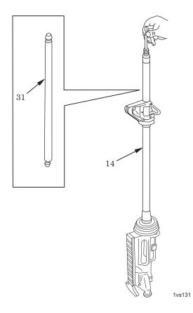
Figure 33. Use of Bore Straightness Gage.
