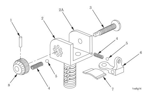
Figure 14. Rear Sight Assembly (M16A2) 9349072 and (M16A3, M16A4, M4, M4A1) 12951026.
