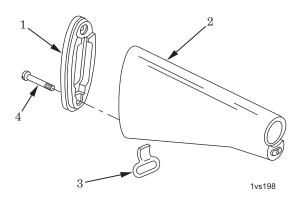
Figure 1. Removal/Installation of Buttplate.
