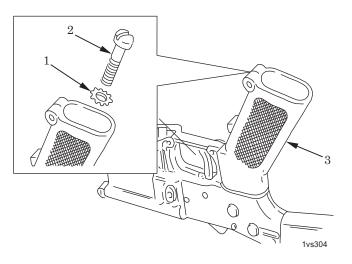
Figure 8. Securing Pistol Grip with Lock Plate Removed.
