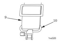
Figure 9. Attaching Sling to Quick Release Swivel.
