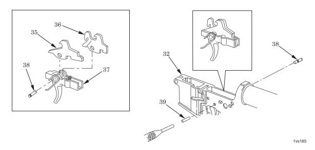
Figure 17. Installation of Trigger Assembly (M16A2/M16A4/M4).
