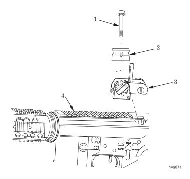
Figure 3. Installation of Back-up Iron Sight.
