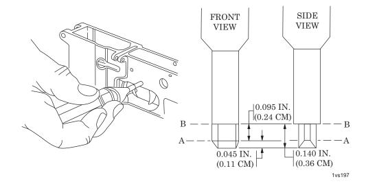
Figure 30. Use of Trigger and Hammer Gage.
