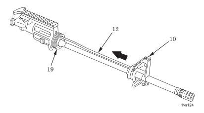
Figure 25. Installation of Gas Tube.
