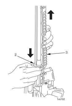
Figure 2. Removal of Lower Handguard Assembly (M16A2).
