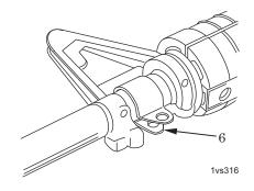
Figure 5. Installing Barrel Band.
