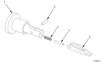
Figure 13. Forward Assist Assembly 9349086.
