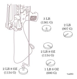
Figure 2. Trigger Pull Test.
