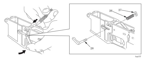
Figure 9. Removal of Magazine Catch.
