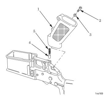
Figure 1. Removal of Pistol Grip.
