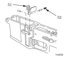
Figure 30. Bolt Catch Inspection.
