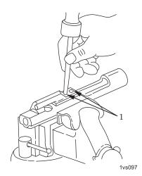
Figure 4. Staking Carrier Key Screws.
