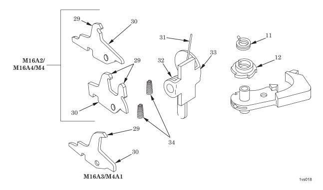
Figure 15. Disconnector, Automatic Sear, and Burst Cam Inspection.
