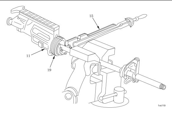
Figure 20. Torquing of Barrel Nut Assembly.
