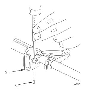
Figure 3. Removal of Small Sling Swivel (Rifle).
