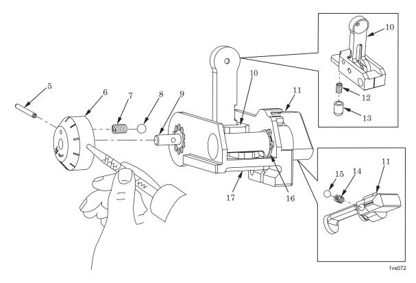
Figure 2. Disassembly/Assembly of BUIS.
