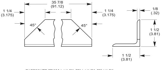
FABRICATE FROM 1 1/2 IN. BY 1 1/2 IN. BY 1/8 IN. ANGLE IRON, NSN 9520-00-277-4902 OR EQUIVALENT. PAINT WITH OLIVE DRAB ENAMEL PAINT, NSN 8010-01-350-5249 OR EQUIVALENT.
