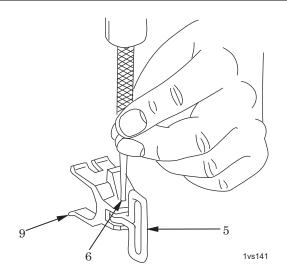
Figure 7. Disassembly/Assembly of Swivel Mount (Carbine).
