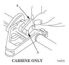
Figure 3. Removing Swivel Locking Bar.
