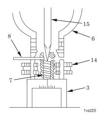
Figure 5. Installation of Helical Spring.
