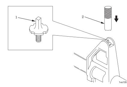
Figure 1. Removal/Installation of Front Sight Post.
