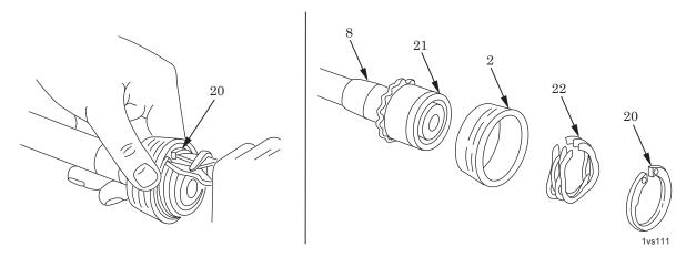
Figure 11. Removal of Handguard Slip Ring.
